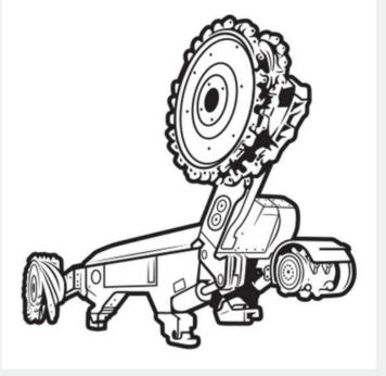
Smart, connected mining machines such as this Joy Global longwall shearer autonomously coordinate with other equipment to improve mining efficiency.
